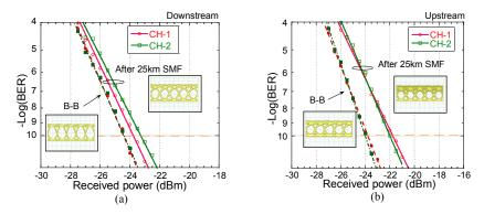
Fig. 4. The measured BER results for 10 Gb/s (a)downstream and (b) upstream transmissions and the corresponding eye-diagrams.
