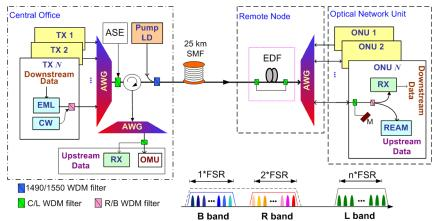
Fig. 1. Bidirectional WDM-PON architecture with channel fault monitoring and a remote pump source.
